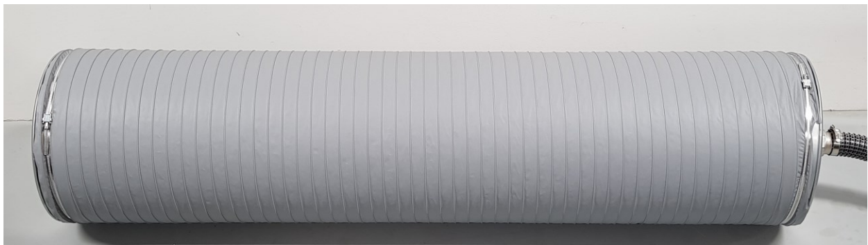
Photo 2: 300 mm flexible hose during gas tightness test
